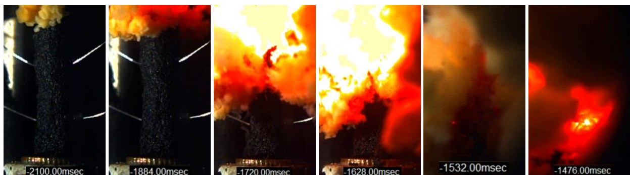
(burning rate 41 mm/s -1 ) P-50 atm
