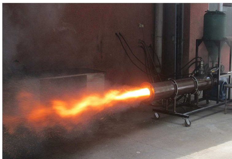
Fig. 8. HRTF torch at PCB outlet during bench testing.
