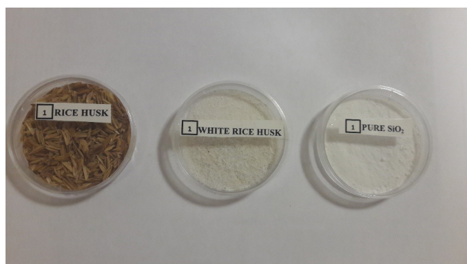
Fig. 3. Appearance of raw rice husk, white rice husk ash and extracted silica from treated rice husk in 2M HCl acid followed by combustion at 600 °C.
