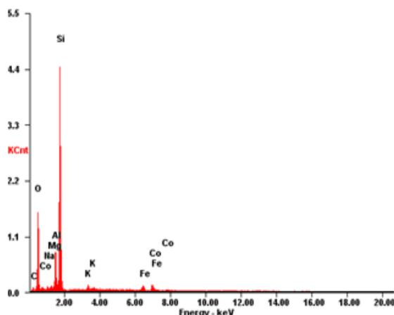
Fig. 5. The EDAX analysis of MWCNT.
