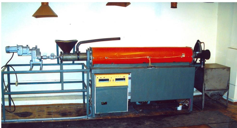
Fig. 1. View of auger furnace for carbonization raw rice husk [16].
