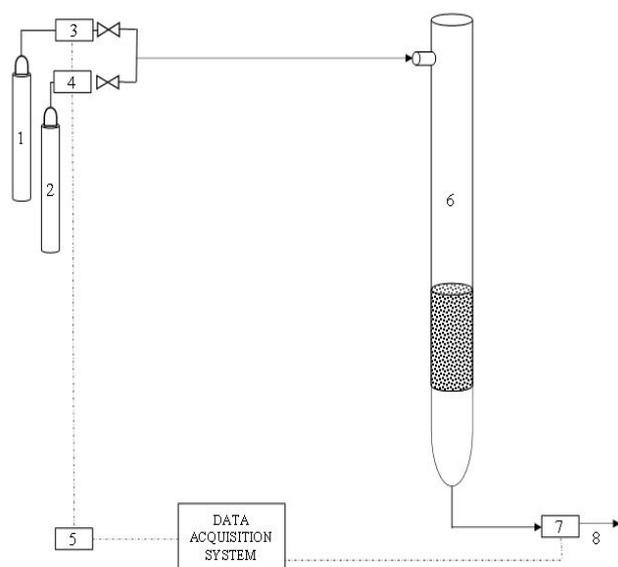
Fig. 2. Experimental apparatus: 1) N<sub>2</sub> cylinder; 2) CO<sub>2</sub> cylinder; 3) N<sub>2</sub> flow meter; 4) CO<sub>2</sub> flow meter; 5) multichannel control instrument; 6) 10 mm ID fixed bed reactor; 7) CO<sub>2</sub> analyzer; 8) stack
